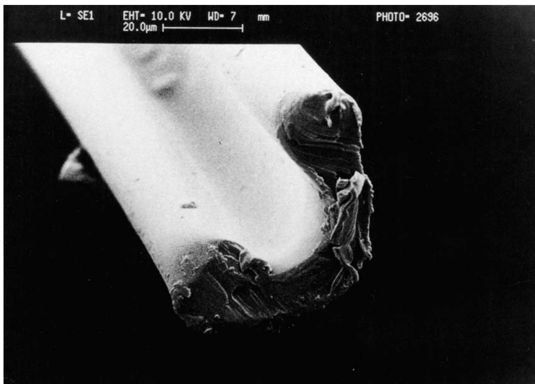
Figure 6 SEM micrograph of dibutylchitin fiber cross section, [\eta] of polymer 1.28 dL/g.
