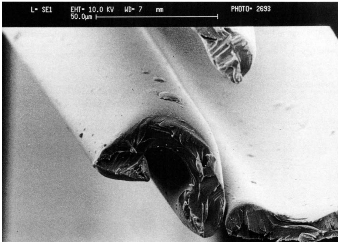
Figure 5 SEM micrograph of dibutyrilchitin fiber cross section, [\eta] of polymer 1.45 dL/g.
